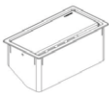
SOCKET BOX 9 POINT ABS 3 ELECTRICAL, 4 LOGIC, USB AND HDMI
